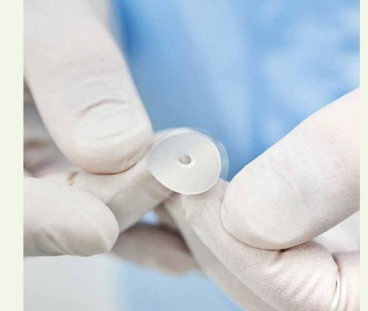
**Protection foil:** Protection of critical areas from Particles and Contamination.
